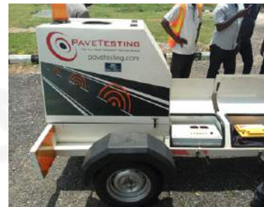
Non-Destructive testing with Falling Weight Deflectometer(FWD) and Becklehem Beam (BB)
