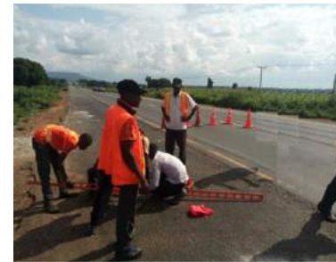
Non-Destructive testing with Falling Weight Deflectometer(FWD) and Becklehem Beam (BB)
